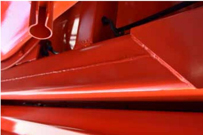
The lower frame is welded from closed steel sections made of high quality construction steel
