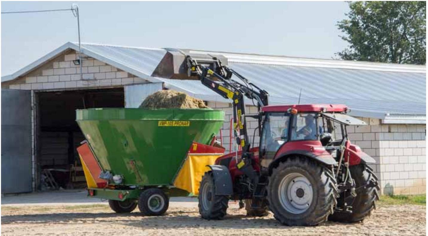
One of features PRONAR mixer feeders have is segmental construction. It allows the farmer to adapt capacity of the machine (even up to 12m<sup>3</sup>) to the size of his herd by
