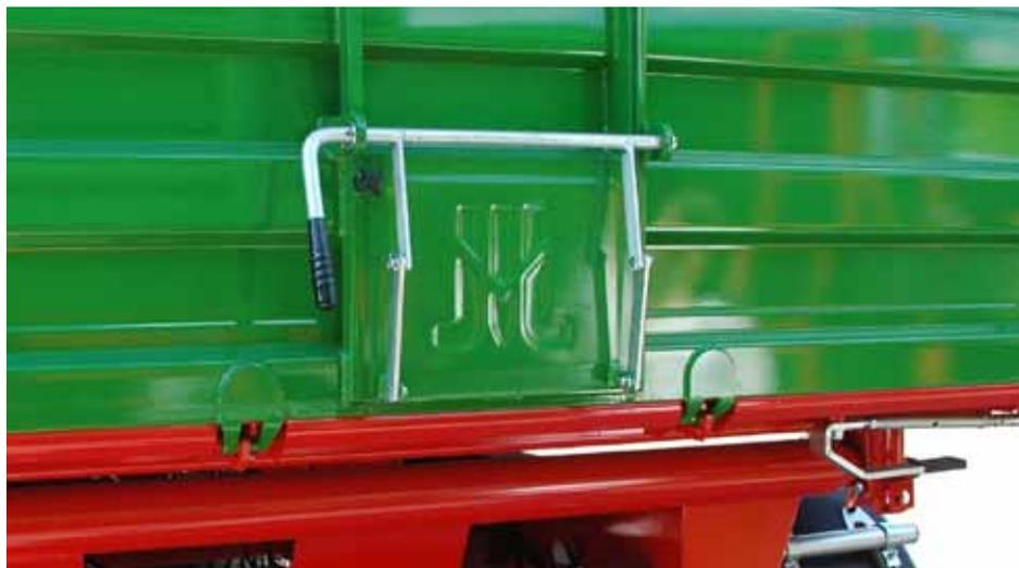
The chute is closed with two tension rods which make it easier to open and lock it.
