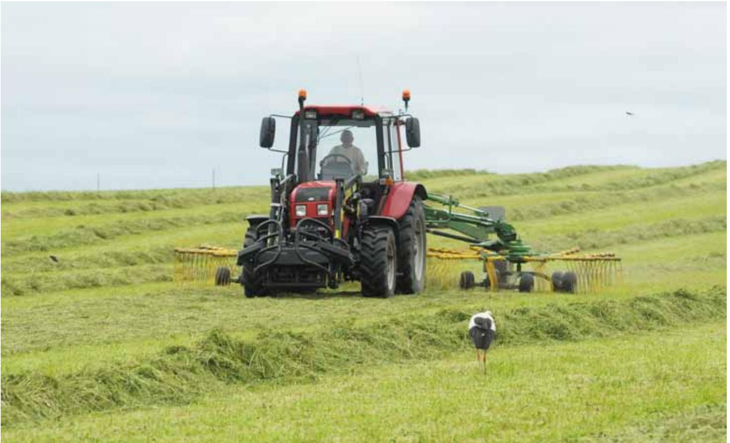
(improving manoeuvrability and ground traction), and two shock absorbers, which improve use comfort. It also has four pneumatic wheels set in tandem. Its intended for use with tractors starting from 22 kW (30 HP). Its mass is 500 kg.
