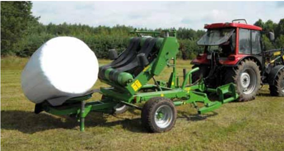
PRONAR Z245 is loaded from the side using a loading arm, while PRONAR Z245/1 is loaded from the front. Each machine counts the rotations of the turntable with a wrapping counter inside the tractor's cab. Depending on the width of the foil, it is recommended to use 24 (for 500 mm foil) or 16 (750 mm) rotations. The wrapped bale is grabbed by the adjustable unloading mechanism and set on the side of the wrapper with the flat side down or is rolled down behind the machine (depending on the model).
