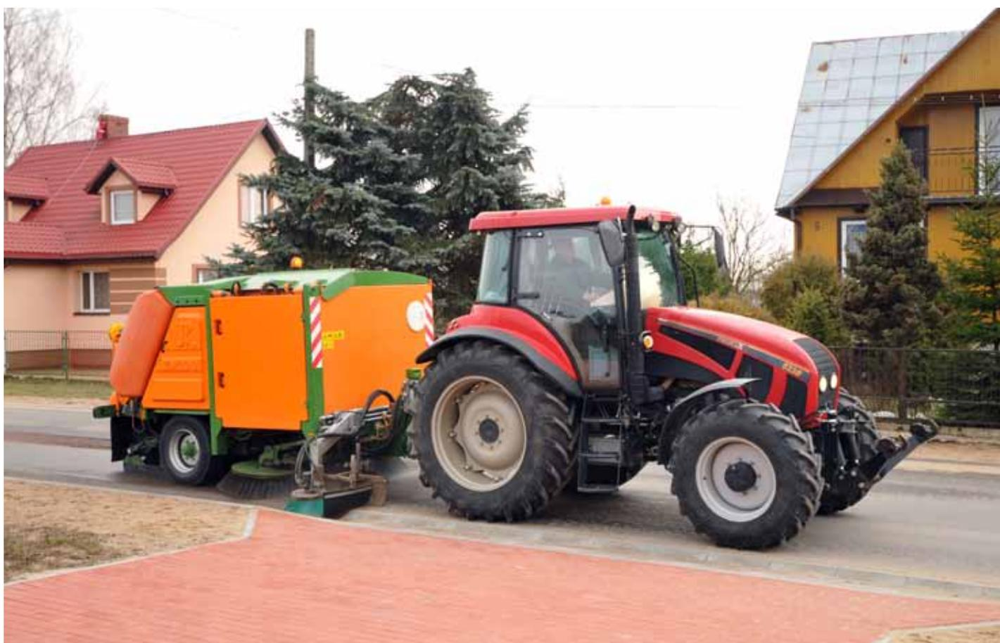
by Pronar's British dealer. The grass-covered surface was cleaned it 95% and suffered no damage after the first pass with minimal pressure set. The surface was thoroughly cleaned and otherwise left intact. Another test positively verified effectiveness of new brushes in gathering up large amounts of wet leaves, a task traditional suction sweepers have trouble dealing with.
