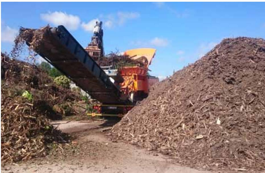
tant indicator of the quality of Pronar machinery. The mobile trommel screener (MPB 20.55) and the mobile slow-speed shredder (MRW 2.85) were combined into a production line to treat varying materials. Effectiveness and smooth operation of these machines astonished even the most sceptic observers and experts.
