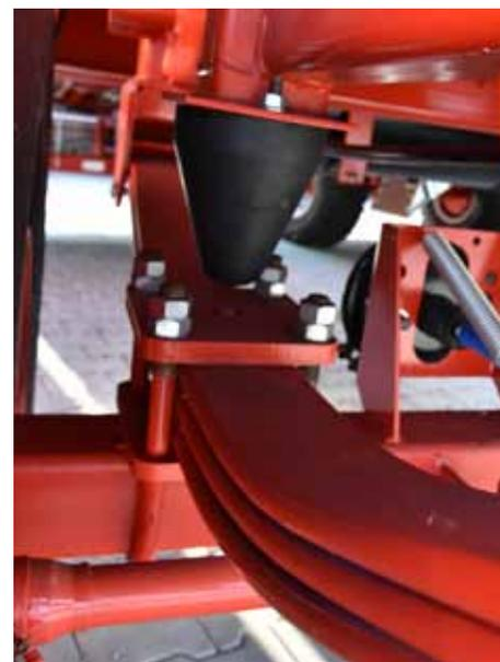
The suspension is based on parabolic springs with three leafs, narrowing towards the end. Thanks to this design they do not require any lubrication.
