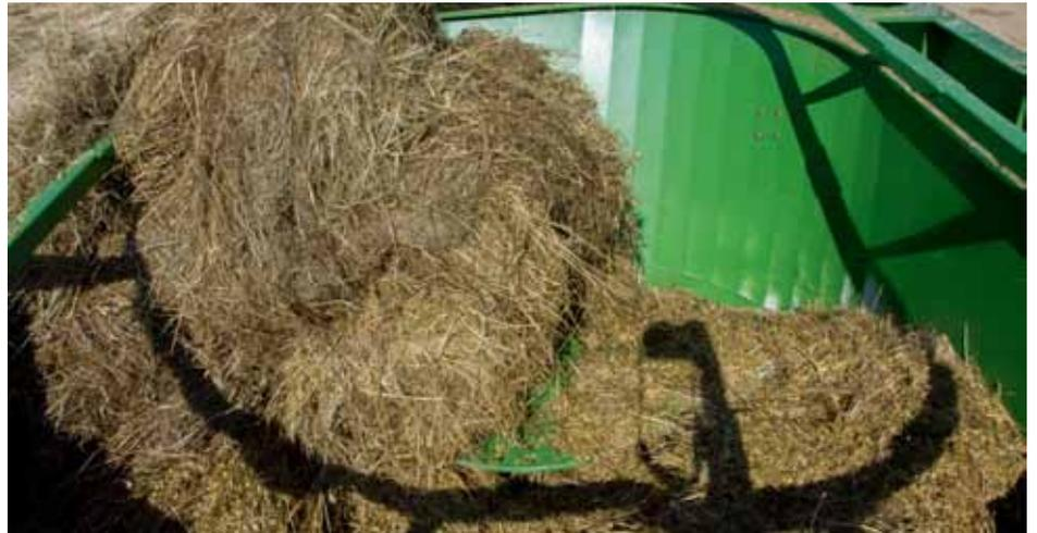
discharge window and one or two side discharge windows (customer's discretion). 250-mm extensions (additional equipment) allow increasing tank capacity to 6m<sup>3</sup>. Rear discharge window is a great convenience for sheds having a narrow passage, as conventional mode of feeding (from both sides of the tank) may result in the feed getting into the drinkers. In larger and broader sheds, two di-
